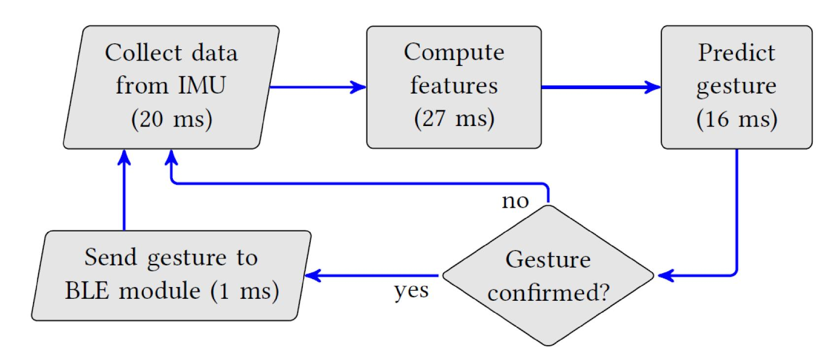
Prediction pipeline loop that runs on the singlethreaded microcontroller (must finish in 100 ms).
